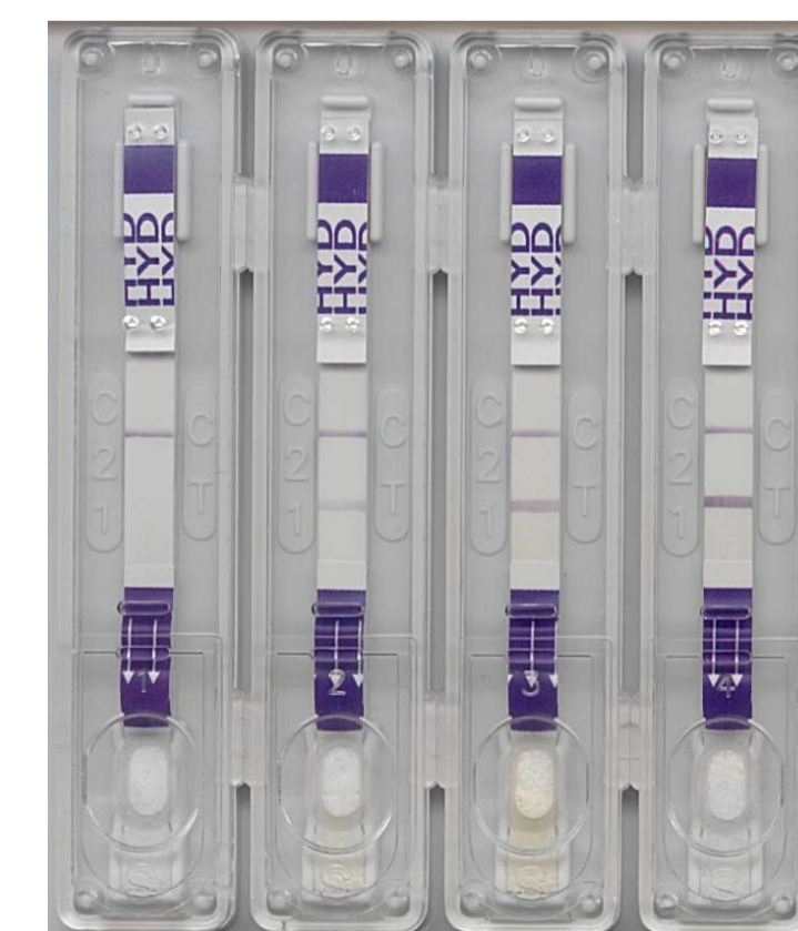
Figure 1. Examples of VIRAPID® HYDATIDOSIS results: negative and positive (low, clear and high) samples.
